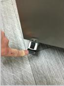
Push your machine 8. to a suitable area and lock the brake lever to avoid the machine
