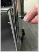
Connect handle to the back of the machine using the 4 wing nuts provided.
