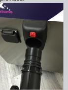
Connect vacuum hose, clicking it into position.Ensure it cannot be pulled out.
