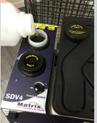
Using clean cold water fill the reservoir and replace cap.
