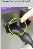
7. Lift the flap and connect the hose ensuring the pin locks into position.
