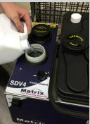
5. If desired. Fill the detergent tank with suitable detergent.
