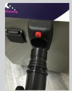
Connect vacuum hose, clicking it into position.Ensure it cannot be pulled out.
