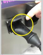
8. Lift the flap and connect the hose ensuring the pin locks into position.
