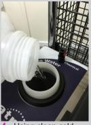
Using clean cold water fill the reservoir and replace cap.
