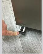
9. Push your machine to a suitable area and lock the brake lever to avoid the machine moving during use.
