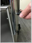
Connect handle to the back of the machine using the 4 wing nuts ovided
