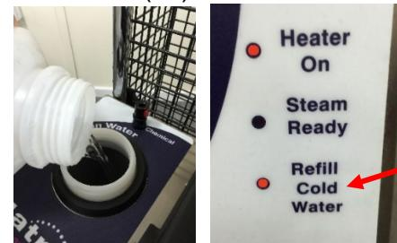
*A buzzer will sound and the steam will no longer come out of the nozzle when the steam switch on the handle is pressed.*
