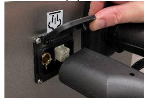
Ensuring it is pushed in all the way and the pin on the flap locks into the hole on the hose.
