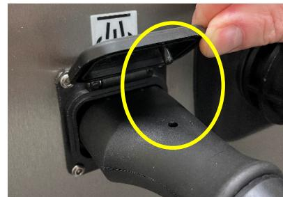
*Ensure the steam hose cannot be pulled out.*
