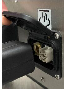
Ensuring it is pushed in all the way and the pin on the flap locks into the hole on the hose.
