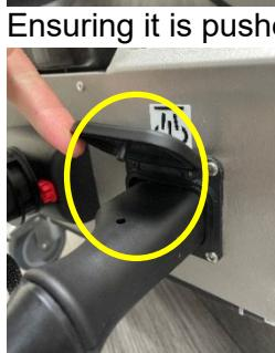
Ensure the steam hose cannot be pulled out.
