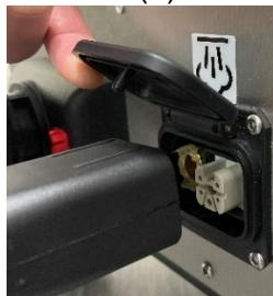
Ensuring it is pushed in all the way and the pin on the flap locks into the hole on the hose.
