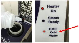
A buzzer will sound and the steam will no longer come out of the nozzle when the steam switch on the handle is pressed.
