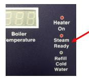
Re-allow the temperature to increase and the steam ready light will re illuminate (9)
