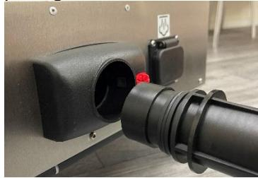
If the Hose becomes damaged the complete hose must be replaced. Do not attempt this task yourself, contact a Matrix approved supplier for replacement.
